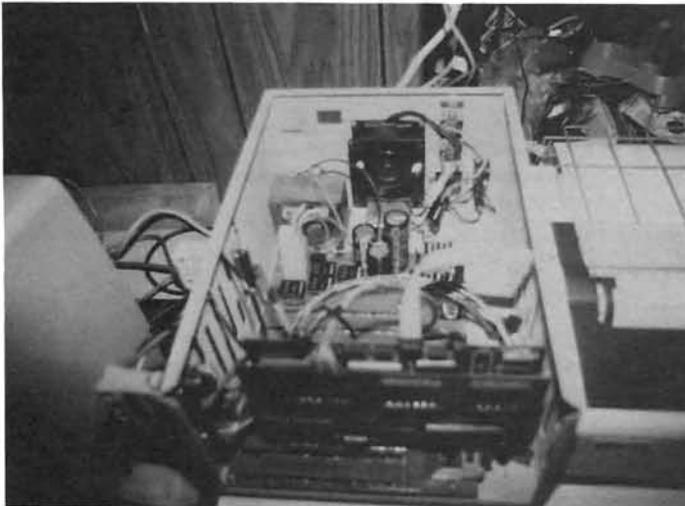
1. The neat and spacious layout of the M89 Expansion Box provides for easy servicing. The entire unit can be dismantled and the mother board removed in less than five minutes.
