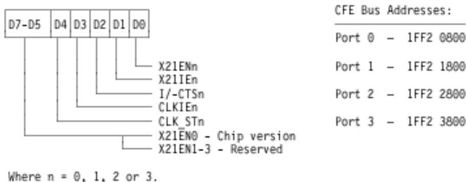
**Figure 13-31. Port n X.21 Enable Register Description**
