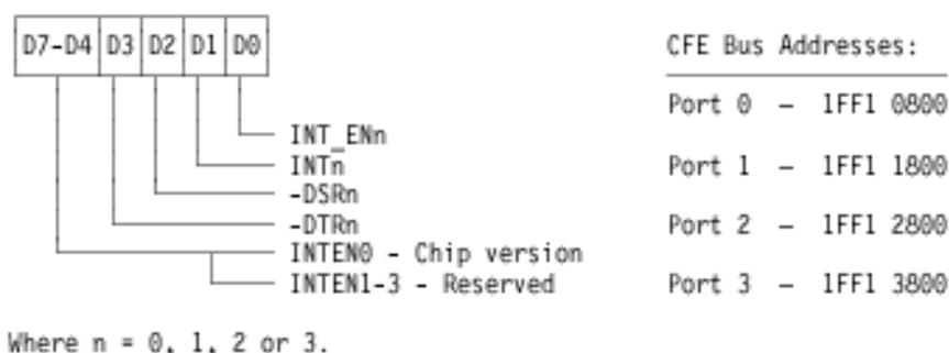
Figure 13-30. Port n Interrupt Enable Register Description
